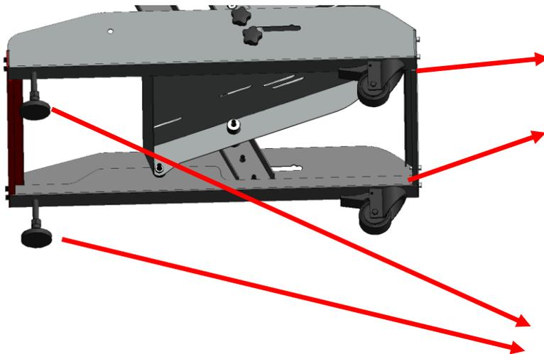
To screw in the castor wheels on the front end, on the underside of the stand, place the threaded stem into the pop nut and turn in the clockwise direction.
