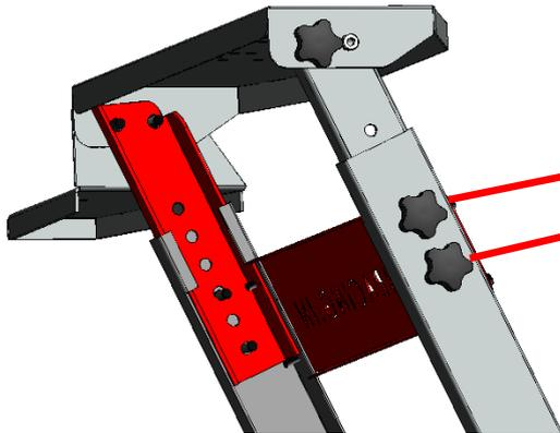
Pull out the 2 flower knobs on either side to increase/decrease height of the steering plate. Tighten the knobs once the steering height is perfect for you.
