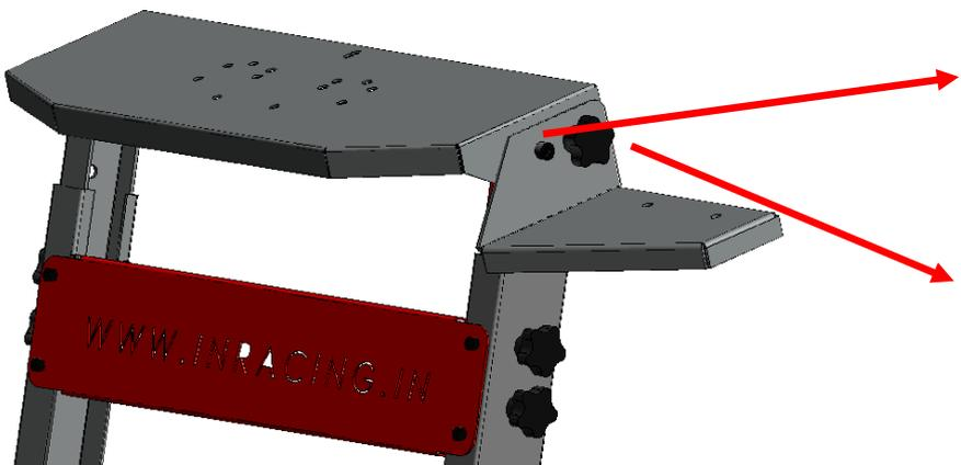
Put the gear shifter plate in place and tighten using M8 Bolt.
